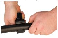
**SLIP** saddle onto pipe BEFORE LATCHING.
