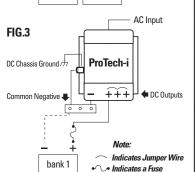
Three Bank / 12 Volt DC Installation (FIG.1) Connect DC cables to three of the positive DC output posts as shown. Connect common ground negative wire (as described below)
