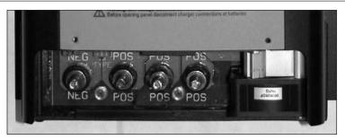
Shown Above: ProTech-i Plus model. The circuit board is clearly marked to identify the polarity of each DC output connection.
