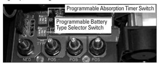
Shown Above - Programmable Absorption and Battery Type Selector Switches. Please refer to page 6 for settings and selections.
