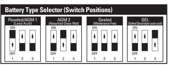
Note: If more than 1 battery type is illuminated, recheck your battery type selector switch positions as illustrated above. It should be noted, only (1) of the 3 switch tabs located on top of the 3 tab dip switch can be in the "ON" position for proper selection and operation.
