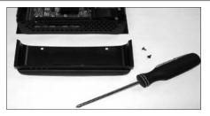
Shown above is the ProTech-i split DC endcap. Please note that this is a two piece end cap. To remove simply unscrew the two self tapping screws on the top of the DC end cap and slide top cap off. This will allow access to the low voltage DC terminals for connections of cables.
